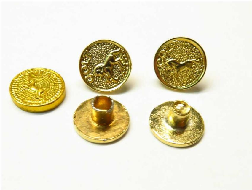
***Some reproduction medallions of different origin. The one to the far left is a simple, glue-in type with an odd, concentric pebble pattern. The other ones look fairly good at first glance, but you can still tell that they are cheap castings. The one in the bottom right corner is so poorly cast that the stem is not even hollow. This means that it can't be staked, and many times you will find these glued in.***
