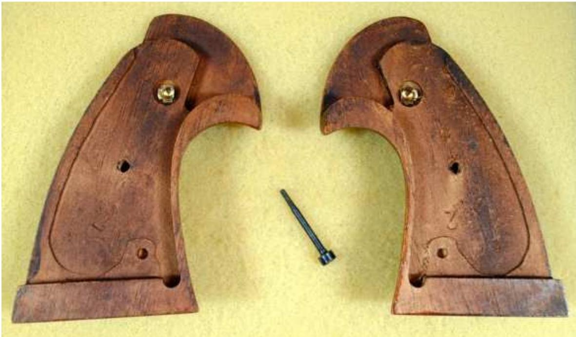
*2nd gen Python grips, back. Note the fitting pads along the rear edges and the pin holes.*
