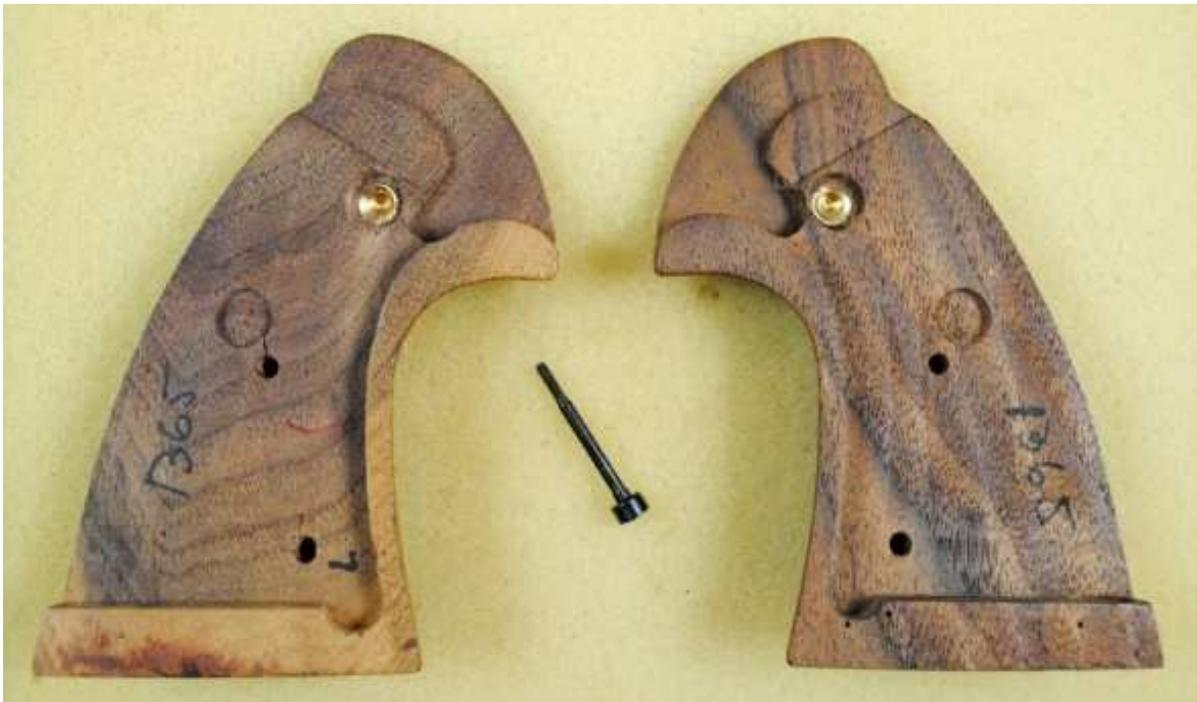
*Late 3rd gen Python grips, back. Note the flat backs, the circular relief cuts for the rebound lever pin and the straight relief cut above the medallions.*
